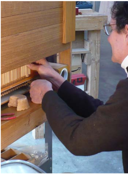
Adjusting the key action, New Positive Organ
