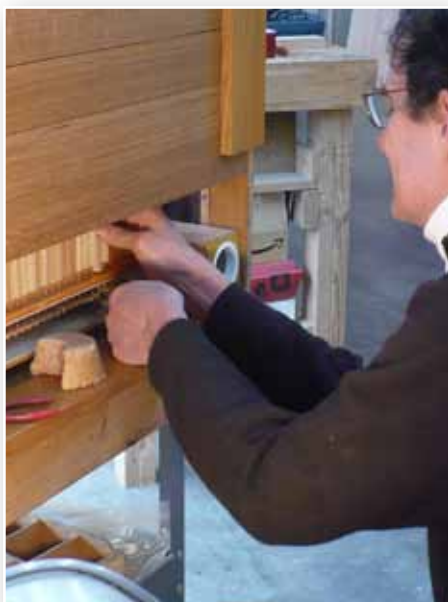
Adjusting the key action, New Positive Organ
