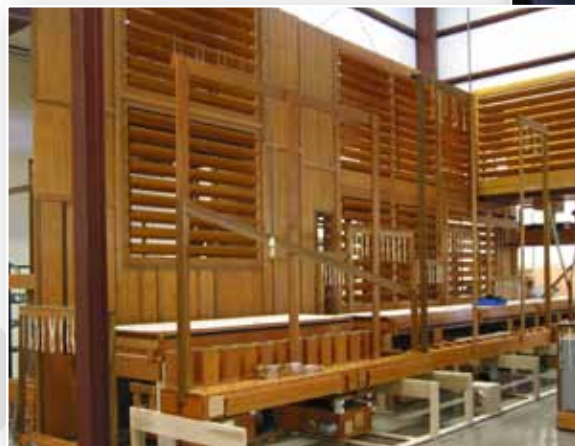
OPUS 1024 4 manual, 103 rank Aeolian-Skinner being renovated in our erecting room and installed in its new home.
