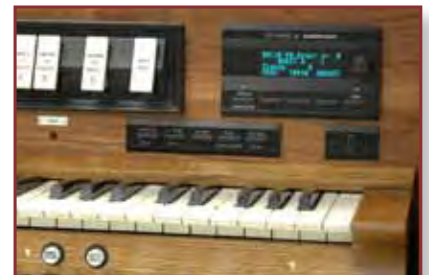
ICS CONTROL PANEL (photo courtesy Berghaus Organ Co)
