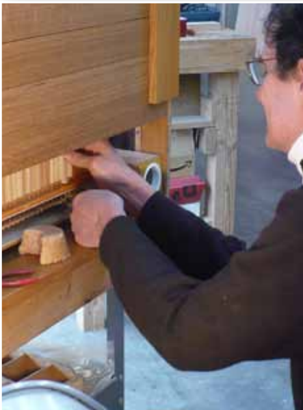
Adjusting the key action, New Positive Organ
